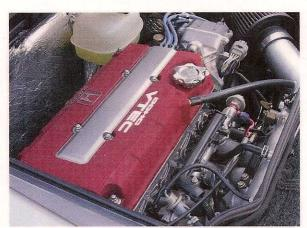
In this new configuration, the rev limiter steps in at a heady 9100 rpm to preempt fragmentation, since the relatively long-stroke Acura engine boasts piston speeds up there in Formula 1 territory.
